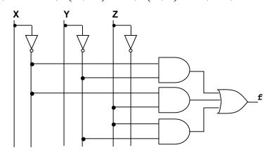
✓  $F = \overline{(\overline{X} + \overline{Y})Z + \overline{X}\overline{Y}\overline{Z}} = \overline{(\overline{X} + \overline{Y})Z}.\overline{X}\overline{Y}\overline{Z} = (X + Y + \overline{Z})(X + Y + Z) = (A + \overline{Z})(A + Z), A = X + Y$  $F = (A + \overline{Z})(A + Z) = A = X + Y$
