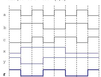
c) The following is the timing diagram of a logic circuit with 3 inputs. Sketch the logic circuit that generates this waveform. Then, complete the VHDL code. (8 pts)
